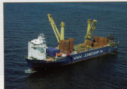
(Below) The ten smallest suction anchors were loaded onto the Jumbo Javelin 's main deck and fastened in the vertical for transportation to site.
